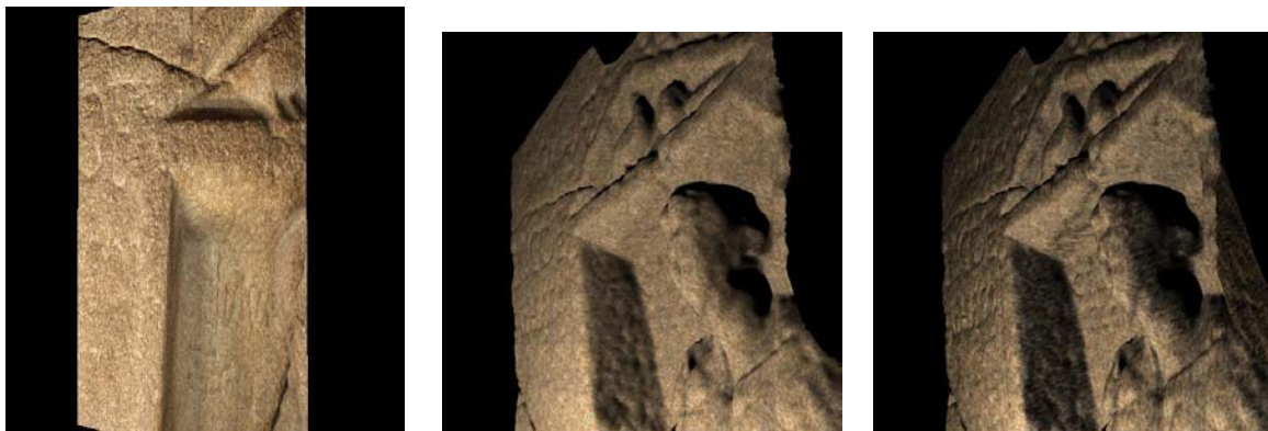
Figure 8: Three snapshots of a façade detail, from a bottom-right viewpoint (left to right): a) a PTM view, b) and c) PBRT rendered views (photo- and PTM-based textured)
