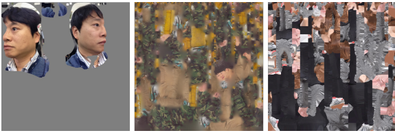
Figure 1: Examples of irregular face textures: Autodesk 123D Catch(left), Agisoft Photoscan(center), and Occipital Structure Sensor(right).
