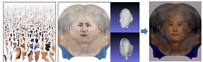
Figure 4: Final texture map (right) generated by the proposed multi-projection approach from the irregular input (left) and the template texture (center) after tone-matching.
