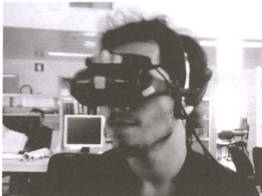
Fig 12 – HMD e sensor de *head tracking*
