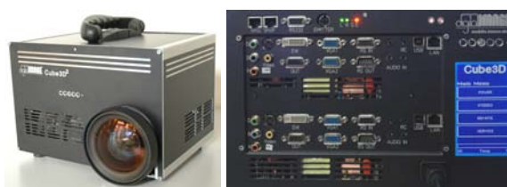
Figure 10: (a) digital IMAGE Series 611 active projector; (b) back with touch panel
