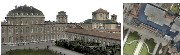
Figure 3: 3D model and High-Resolution Orthomosaic of Reggia di Venaria generated via UAS and processed using the commercial software Agisoft Metashape Pro.
