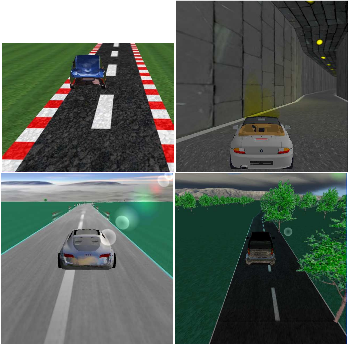
Figure 4: Some clients developed by the students. (Top-Left) Dynamic reflections on the car. (Top-Right) Projective texture for headlights and tunnel lamps fakes with textures. (Bottom-Left) Motion blur and lens flare. (Bottom-Right) Billboarding for showing trees.
