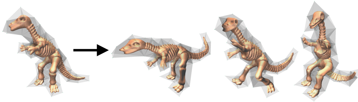
Figure 7: Surface deformation via tetrahedral subdivision. Initial shape shown (left) and three deformed poses (right).
