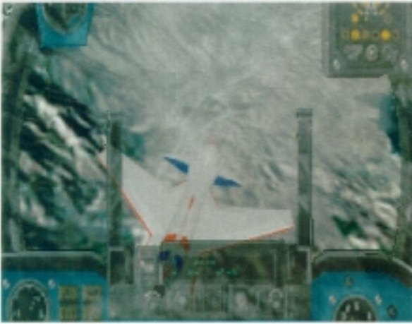
Figure 1: A flight simulation scene mixing a texture-mapped polygonal terrain, an opaque plane (with 4420 polygons), a translucent cockpit, and a volumetric cloud.
