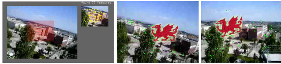
Figure 1: Augmented reality in videos based on SURF descriptors. The user selects an area in one frame (left image). The object, the dragon, is superimposed on that area (middle image). The object is then replicated to the other frames of the video in the same position and rotation as it was when placed (example frame in right image).
