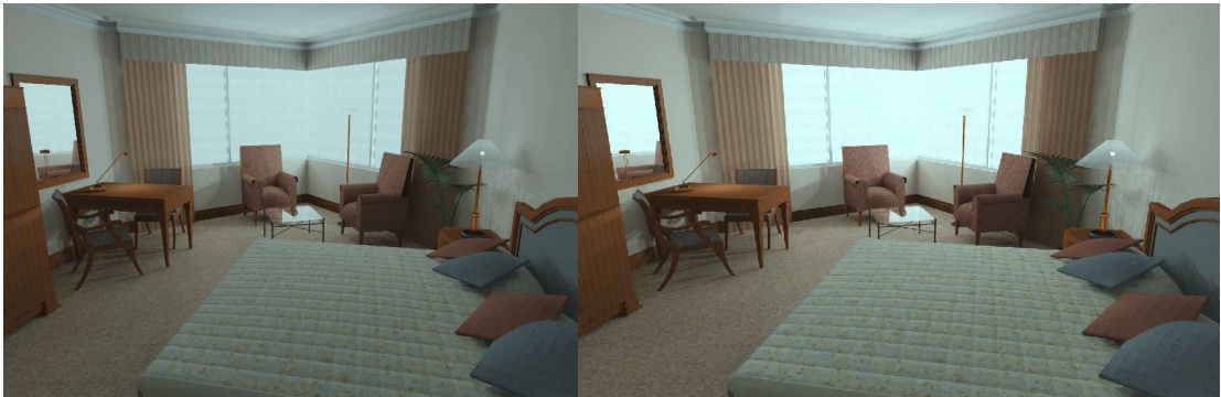
Figure 8.3: Hotel room [Crone, Fowler and Kerrigan 97] (3000 x 1950); image obtained with our operator but without added the glare (left), image obtained with our operator with added the glare (right). The original image has luminance range equal to [0.37; 18828] \text{ cd/m}^2 .
