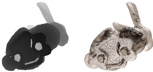
Figure 5: Reconstruction from a holed model results in an excessive carving inside the shape. The depth image of the Bunny model shows missing data in its base (lighter colors denote farther points). On the right, the isosurface shows a set of cavities given by the depth carving.
