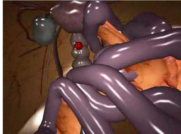
Figure 11: Example application of collision detection (intestine surgery simulation). The objects in this case are highly deformable. Both self-collisions and collisions between different objects must be detected and handled. (Screenshot courtesy L. Raghupathi, L. Grisoni, F. Faure, D. Marchall, M.-P. Cani, C. Chaillou [RGF*04].)
