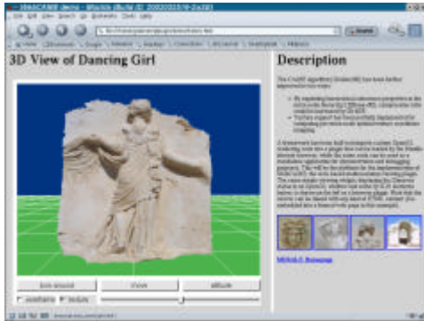
Figure 19: Viewing window with LOD processing embedded into a framed web page as a browser plugin
