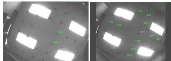
Figure 3: Ability of VGA (left) and XGA (right) InertiaCams to decode 12.7 cm fiducials from 2.7 m distance
