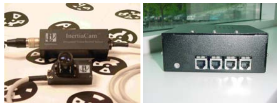
Figure 1: First Generation VisTracker, comprising InertiaCam sensor head, InertiaCam electronics unit, and wearable Sensor Fusion Processor
