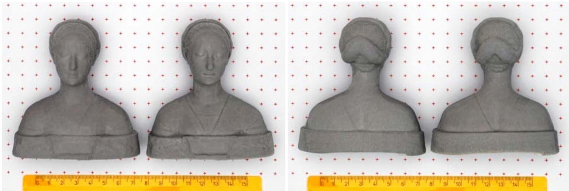
Figure 5: The color-enhancing technique in action on the Laurana model. Represented objects are less than 10 cm tall (crosshairs are 1 cm spaced). In each pair of images, the left model is a standard uniform color reproduction, while on the right the same 3D model have been printed with enhanced color: many small details whose shading is canceled by the SSS are again visible in the model on the right.
