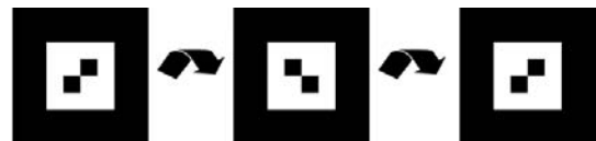
Figure 4: This marker matches itself after two rotations by ninety degrees.
