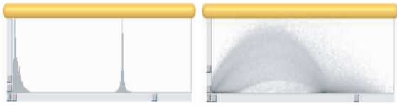
Figure 1: Histograms are useful in classification and are often displayed as the backgrounds of transfer function editors. Here we see a 1D editor/histogram (left) and a 2D editor/histogram (right).
