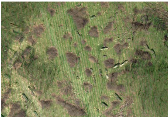
Figure 6: Zoomed view of 3D point cloud and orthophoto after application of the threshold value. Most clearance and even wood piles are filtered out and are not represented in the point data any more.
