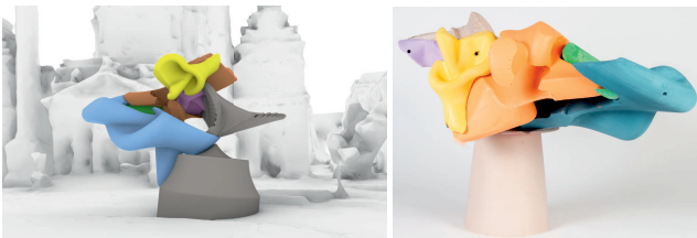
Figure 14: Visualization of the Nuloid (left): The six links of the invertible paradoxical loop have different colors, where the base-link (including the grounding structure) is gray, and the end-link is orange. Model photo of the Nuloid (right).
