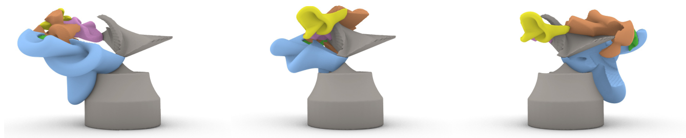
Figure 1: Our interactive tool allows the user to design invertible paradoxical 6R loops, which are free of self-collisions.
