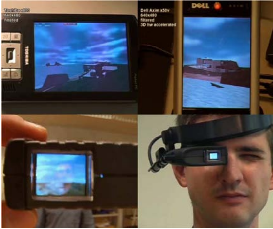
Figure 3: Test scene rendered in realtime on the e800 and x50v embedded screen and on the head-worn display.
