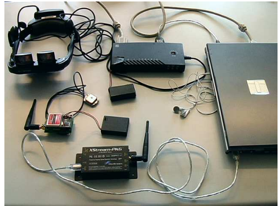
Figure 1: Required equipment for a typical wearable Augmented Reality framework: a notebook, a stereographic see-through HMD, a GPS antenna, some battery packs.
