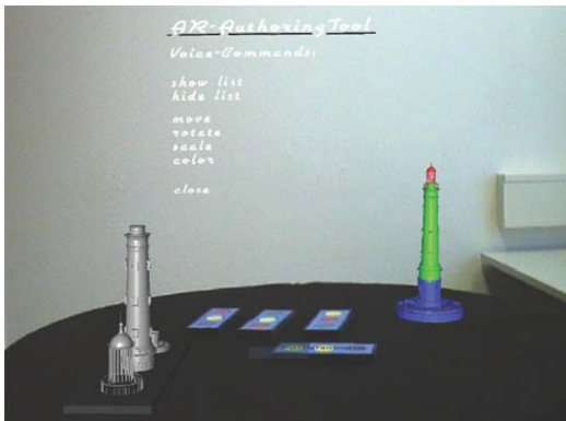
Figure 2: The augmented voice-command list in the user's eye level and the activated 3D content repository
