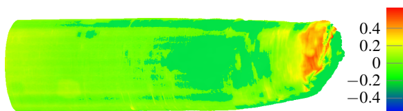
Figure 11: Aligned \mu CT mesh with our reconstructed point cloud colored according to the Euclidean distance. Distances are in mm.
