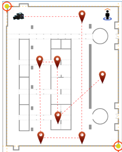
Figure 5: Example of a camera path generated in the 2D editor over a loaded scene. The initial point is displayed as a camera and it is connected by a discontinuous line to the remaining route points.
