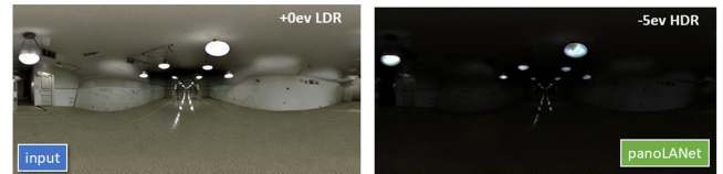
Figure 4: HDR panorama reconstruction using PanoLANet [YLL*21]. Left: input panorama at 0 EV (normal exposure). Right: PanoLANet's reconstruction, retaining more light information at -5 EV. This allows our technique to extract the relevant radiance information for our emissive mesh.
