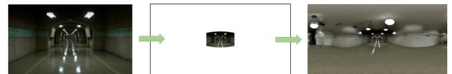
Figure 3: Left: LFOV input image. Middle: equirectangular projection of input (fov is 72°) and visibility mask. Right: LDR panorama reconstruction using PanoDiff [WCL*23] diffusion model for photorealistic panorama outpainting.
