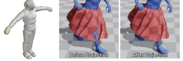
Figure 6: We fit capsules to each joint of the character and use them as collision geometry to adjust for visible intersections in the final render. A typically example of this fix is shown above.
