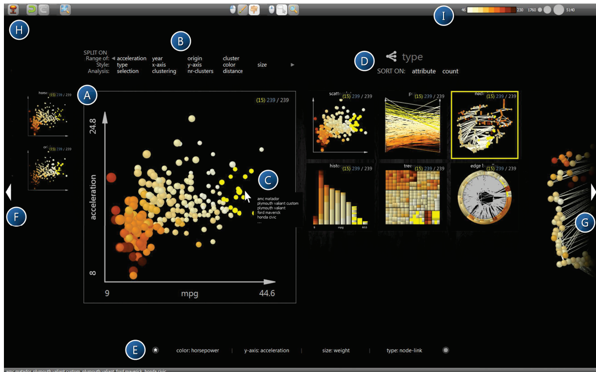
Figure 4: Graphical user interface: The menu (B) on top of the large single (A) shows different parameters that can be selected to produce small multiples. Hovering over the menu items provides information on the current value such as what attribute is mapped to color, or what is shown on the x-axis for example. (C) Items are highlighted across all visualizations, identical to standard brushing and linking mechanisms in multiple coordinated view systems. A user-adjustable radius around the mouse cursor determines what items are highlighted. The number of highlighted items in the current visualization is shown in the upper right corner, along with total number of items in the visualization and total number of items in the data-set. (D) Information on parameter that is split on. Also, multiples can be sorted based on parameter value or number of items contained in each small multiple. (E-G) Navigation mechanism to explore visual history trail. (H) Undo, redo and reset exploration options. (I) Legend with color and size information of small multiple visualization currently hovered.
