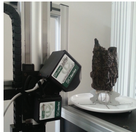
Fig. 5. Test sample positioned on top of a control object (see below test sample) and on a rotating stage to automate the 3D scan acquisition phase.
