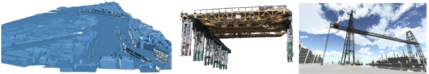
Fig. 3: Use cases' 3D models with different acquisition techniques : 3D scan, photogrammetry, and 3D reconstruction (CAD model).
