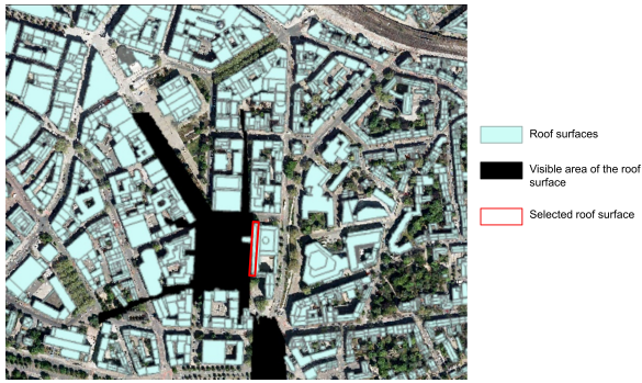
Figure 3: Result of the visibility analysis for one selected roof surface in the study area in Hanover.
