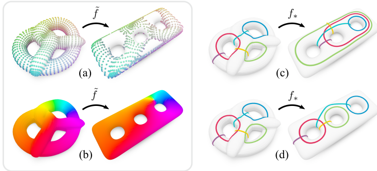
Figure 5.12: Due to non-surjectivity and severe misalignment in the input \tilde{f} (a), the interpolated mapping of periodic potentials (b) may yield non-closed 1-forms. In such cases, an integral-based homology inference via (5.15) may fail (c) as it considers integrals along representative paths only; the global similarity-based inference (5.16) can compensate for such errors and yields the expected result (d).
