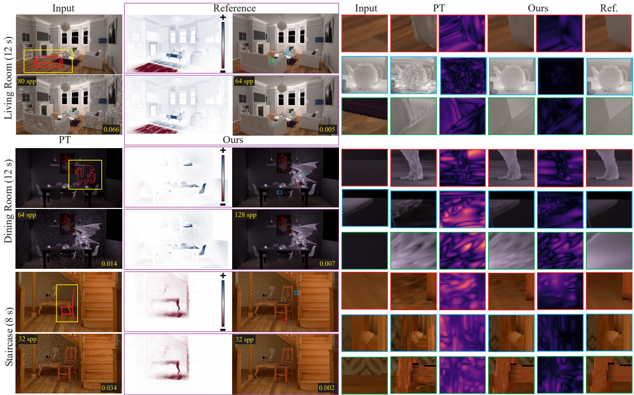
Figure 5: An equal-time comparison for object insertion achieved by adjustment of spp values. Only the indirect illumination is displayed. Rows: Three different scenes. Columns: First, an unmodified input scene above the PT solution. Second (in purple boxes), the reference solution and its difference to the input above our solution and its difference to the input. Finally, three zoom-in crops (rows) for the input, PT, Ours and Reference along with FLIP error maps w.r.t. Reference. The yellow numbers show the RMSE.
