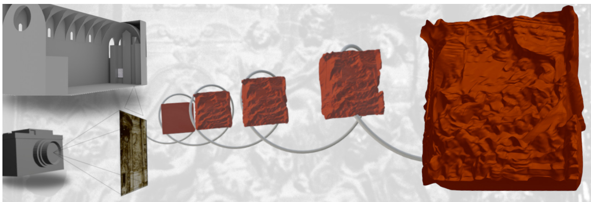
Figure 1: Using a historical photograph of an altarpiece and knowledge of its original context (left), we can determine the camera position and create a lighting environment map. With this information, we leverage differentiable rendering to generate a 3D model that represents the volumes shown in the historical photograph (right).
