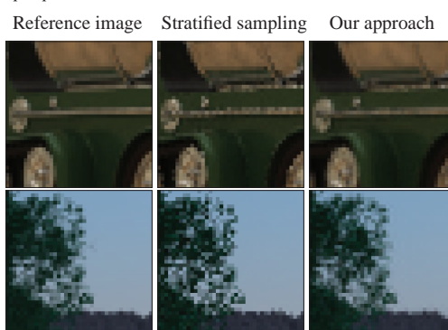
Figure 4: Comparison to reference image. Insets from the TRAIN image (top) and the GARDEN image (bottom) compare traditional stratified sampling and our approach at 4 samples/pixel to a reference image, rendered at 16 stratified samples/pixel.
