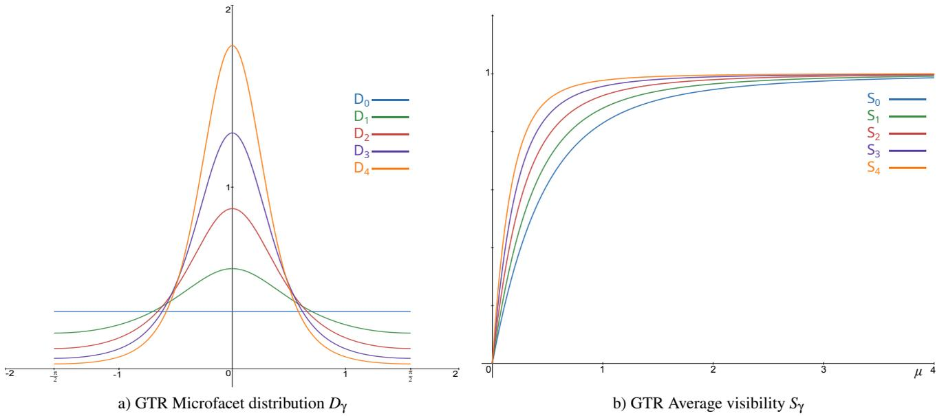
**Figure 9:** Plots of the microfacet distribution  $D_\gamma$  and the average visibility  $S_\gamma$  for  $\gamma = \{0, 1, 2, 3, 4\}$  and for a fixed roughness  $\alpha = 0.6$ . Note that  $\lim_{\alpha \rightarrow 0, \gamma > 0} (D_\gamma, S_\gamma) = (\delta, 1)$  and  $\lim_{\alpha \rightarrow 1} (D_\gamma, S_\gamma) = (D_0, S_0)$ .
