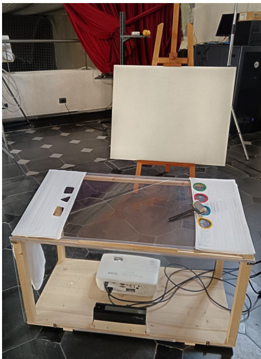
Figure 1: The CambiaColore system set-up. The picture shows the table, the projector, the Kinect camera, and the paint roller used to interact with the system. The drawings created through CambiaColore are projected onto the white canvas facing the table.
