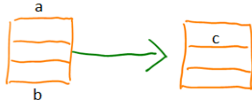
Figure 3 Stroke a and stroke b are Class Connected. Stroke a and stroke c are not Class Connected as there is an edge stroke dividing them.
