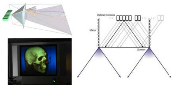
**Figure 1: Light field display.** The light field display is composed by an array of projectors densely arranged in an horizontal array behind the screen, all of them projecting their specific image onto the holographic screen to build up a light field.
