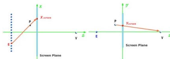
**Figure 2: Light field geometry:** Left: horizontally, the screen is sharply transmissive and maintains separation between views. Right: vertically, the screen scatters widely so the projected image can be viewed from essentially any height.
