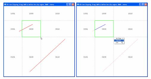
Figure 2. A clipping rectangle is defined by dragging the cursor. Resulting clipped lines.
