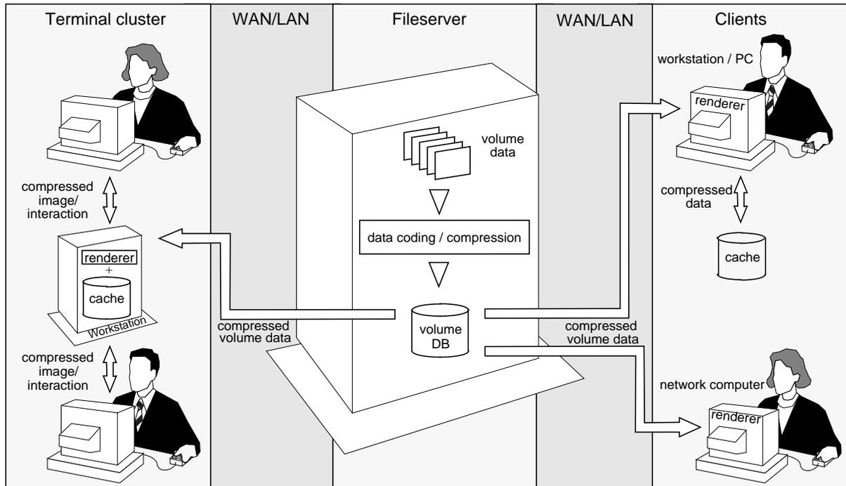
**Figure 1:** Volume-rendering in a distributed client/server environment.
