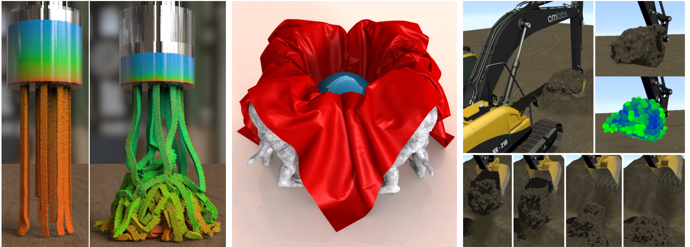
Figure 5: Various examples of constraint-based material simulations. Left: A plastic material resembling modeling clay is pressed into strings and piles up on the ground [YLL*24]. Middle: Realistic wrinkles form on a position-based elastic cloth being pushed down by a heavy object [BKCW14]. Right: Coupled real-time simulation of an articulated excavator, modeled as a stiff multibody system, interacting with position-based cohesive soil [HG18].
