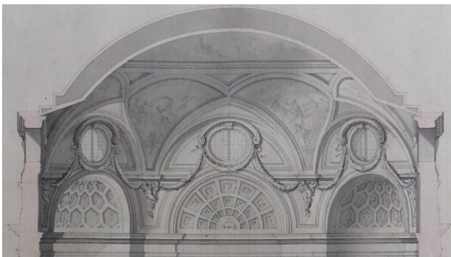
Figure 10: Close-up of ASCB, 1238A, fD ( Fig. 7 ). See the discontinuity between the central portion of the vault and the lunette.
