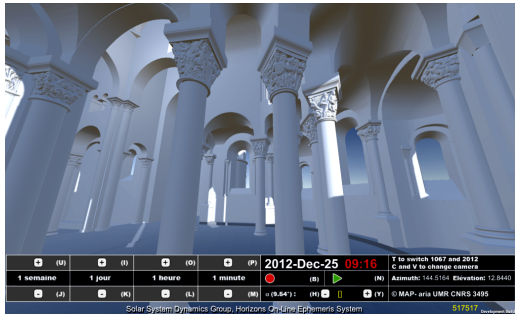
Figure 8: Desktop implementation of the digital heliodon.
