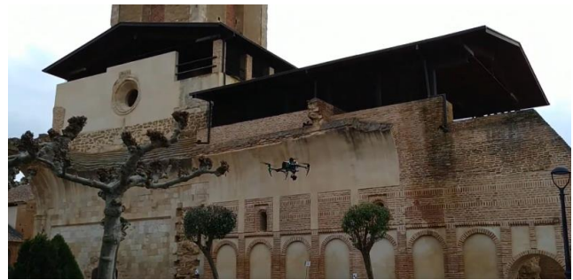
Figure 3: Data acquisition for aerial photogrammetry using a DJI Inspire 2 drone.
