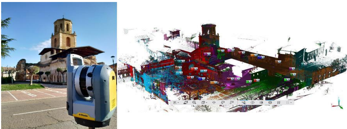
Figure 5: (Left) Trimble X7 laser scanner used for digitizing the exterior spaces of the monastery. (Right) Resulting point cloud after aligning all exterior scans.
