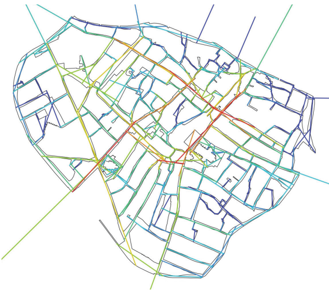
Fig. 4. Integration values (radius n) of the Space Syntax Analysis on the 1529 street layout of Vienna
