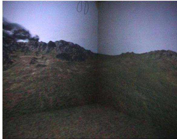
**Figure 4:** Mountain scene (15727 triangles) displayed on a CAVE. The scene is rendered with shadow mapping, multi-texturing (9 layers), 4 normal mapping passes, and screen-space ambient occlusion.
