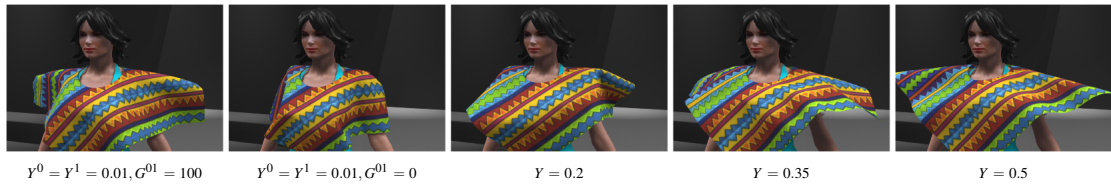
Figure 4: Shear vs. no bending shear: a high bending shear modulus tends to align folds and wrinkles to the material axes (leftmost); a lower shear modulus allows the fabric to fold along other directions, and therefore to obtain a closer fit to the body (second frame). Shearing effects cannot be reproduced by simply tuning Young moduli (3 unsuccessful attempts shown on the right).
