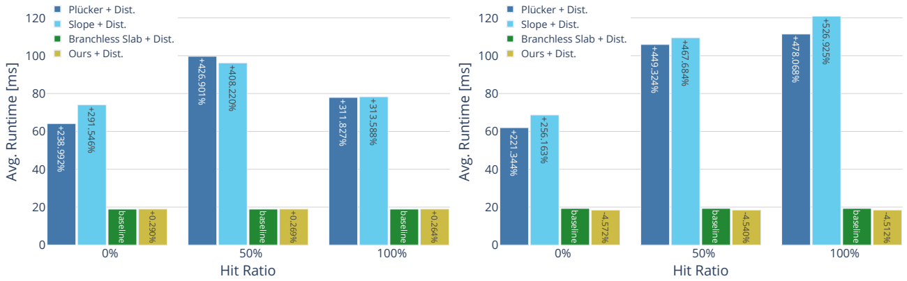
Figure 2: Performance results for g++12.3.0 (left) and clang-15.0.7 (right) with -march=native , with intersection distances. Relative performance to the optimized branchless slab test (baseline) is noted in the bars.
