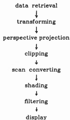
This structure is reflected by the internal structure of the CIG system (Fig. 1). There exist some subsystems arranged in pipeline, doing the above mentioned task.
