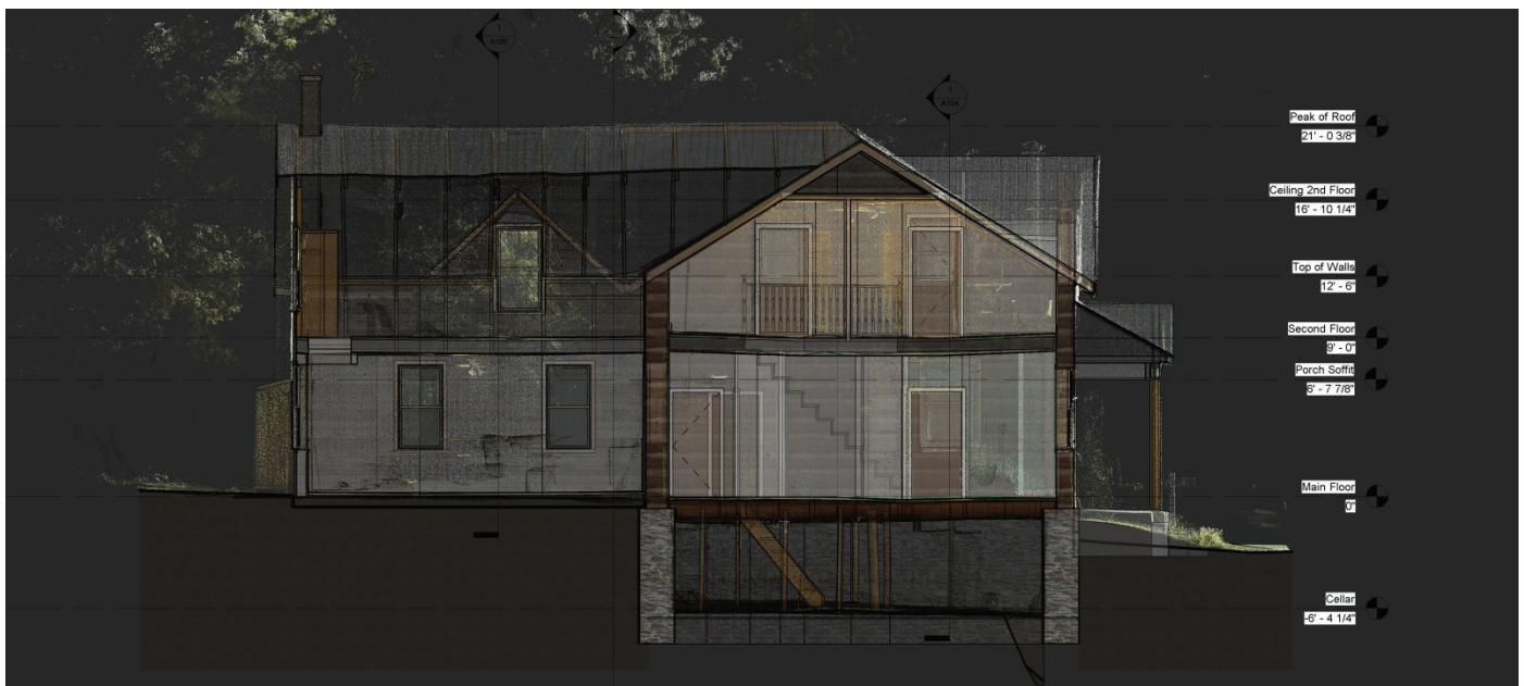
Fig. 1. Longitudinal Section in Revit 2014 showing / Frame Building BIM and pointcloud.
