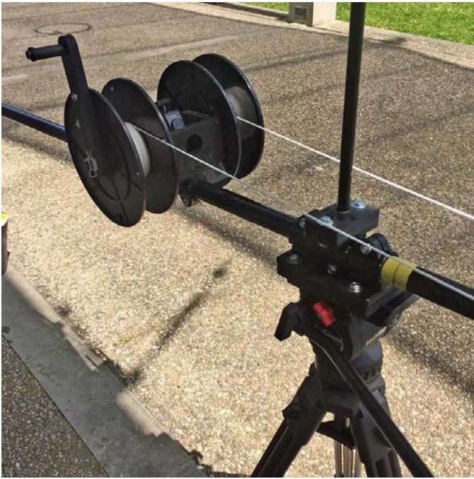
Fig. 4. The central mechanism, partly made of carbon rods and printed and/or laser-cutted frames
