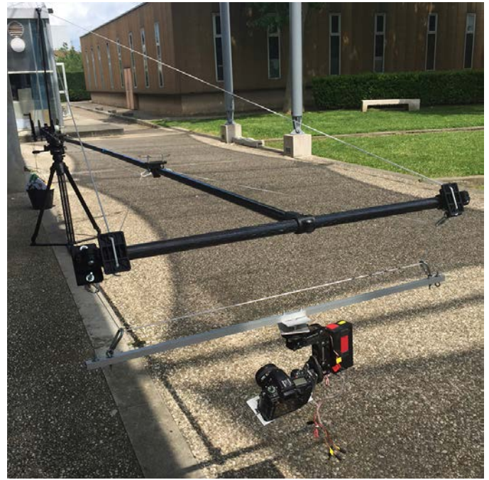
Fig. 5. A close view of the suspended remote-controlled camera mount (tilt and yaw action).
